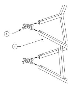
**3.** Continue to insert the crosspieces (4) into the other two brackets (1). Secure the brackets (1) to the crosspieces (4) by using the 16x screws. Please note the position shown in the diagram.
