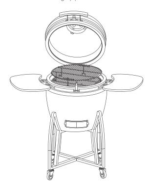
Carefully pull the grill when moving. To prevent the potential of grill tipping it over, never push grill. When the grill is in the desired location, push down the tabs on the locking casters to set the locks.
