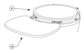
**12.** To attach the handle (11) to the lid of the Kamado Grill (9), use the 2x pre-attached bolts with their corresponding washers, locking washers, and nuts per bracket.
